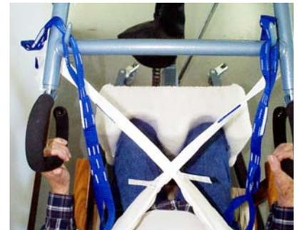
View from above the VERA-LIFT™ showing the Crossed Strap Method of connecting the back belt to the lift
